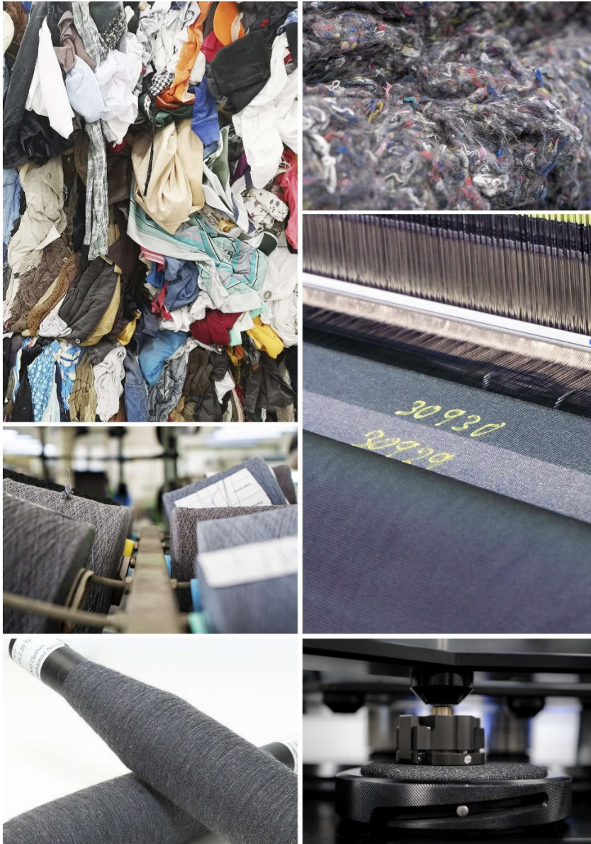
Image 1: The mechanical recycling process enables the re-use of blended fibers from old clothes, in form of high-quality yarns. (Credits: imat-uve)
